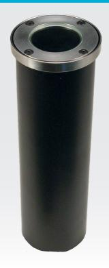
Precision machined LED lighting fixture with 12V input LED Light Engine (COB with integrated driver module). Modular industry standard components allow for simple field replacement and future upgrade. Designed for in ground wet location installation for up lighting trees, landscapes, or any vertical hardscape / architectural surface.
